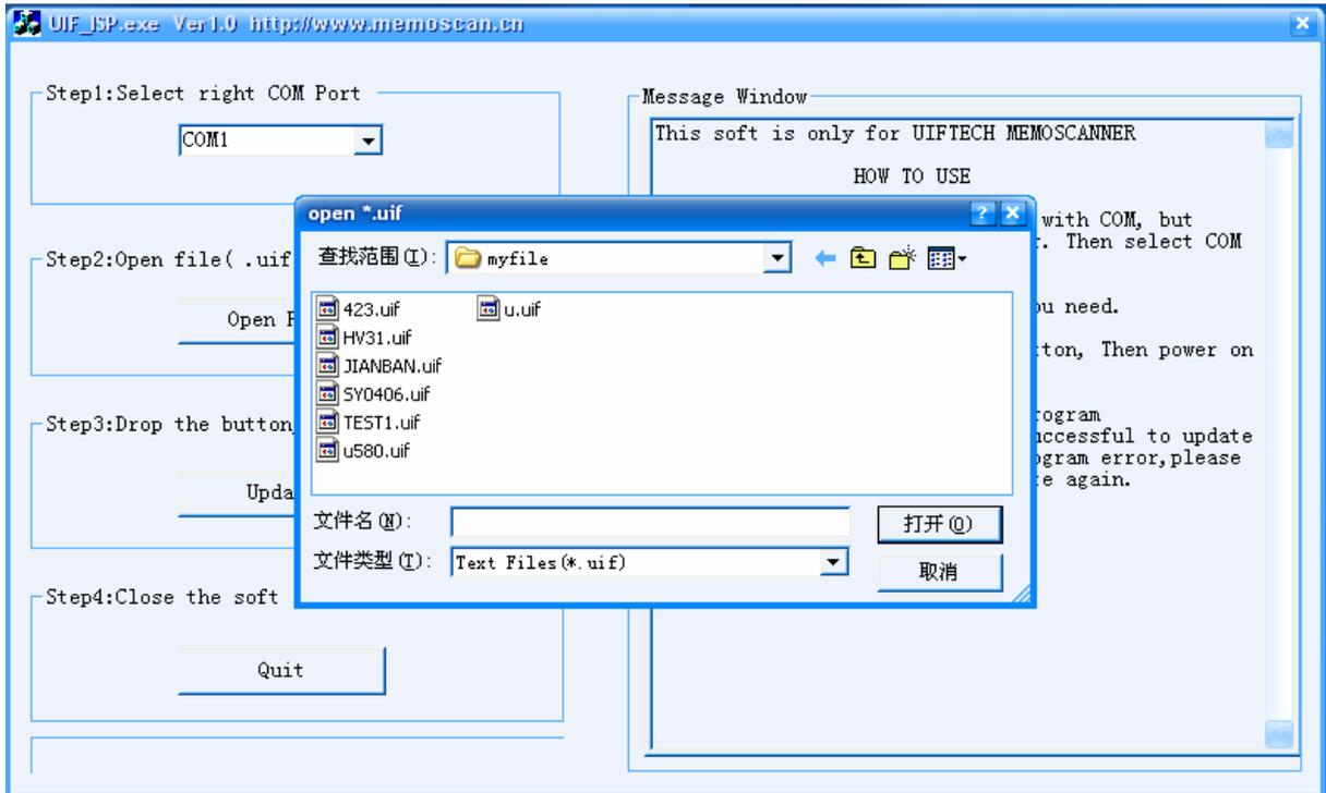
4. Press "update", open the power of memo scanner, there will be the interface as follows. The Memo scanner is trying to connect with PC.
