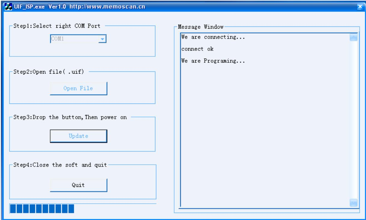
5-1. If the below interface appears in the process of upgrading, that's to say the communications failures, this time requests to close the procedures and re-run the programmer
