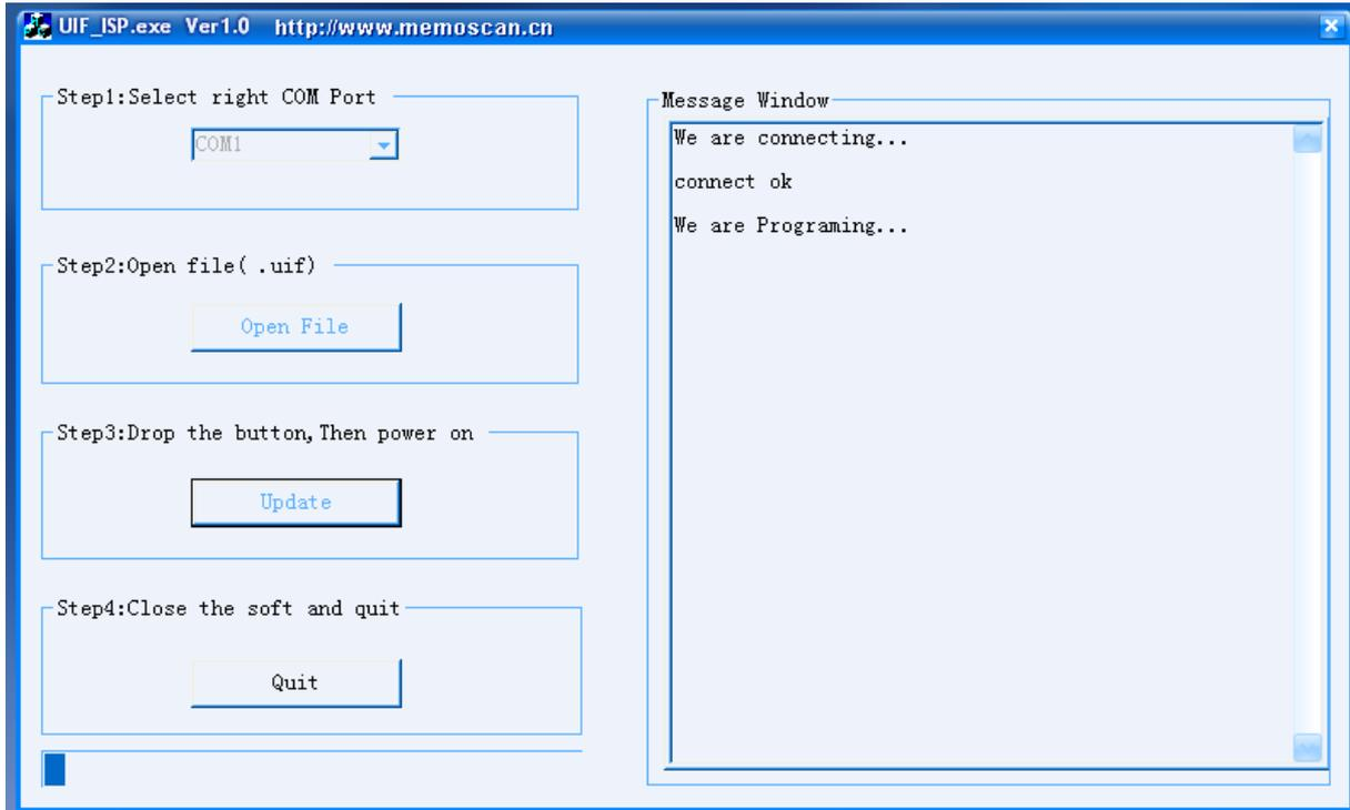
4-2. If the connection is fail, this time requests to close the power of memo scanner and check whether the connection and the choice of COM mouth are right or not.
